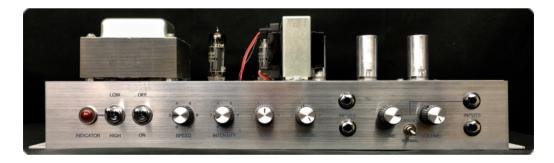
controls. The other channel has Volume, Tone and Tremolo with Speed and Intensity controls. Also on the front panel are the On/Off switch, a Standby switch with High and Low power switching, a NORMAL/CASCADE switch and an On indicator lamp.
