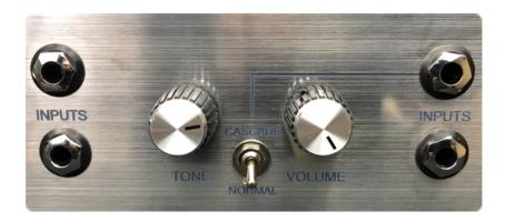
the CASCADE position. What it does is route the signal of Channel 1 into the input of Channel 2 (with some additional tone and gain shaping parts to make it sound best) giving you more gain. When you are plugged into Channel 1 and the front panel switch is in the CASCADE position, both channels are active and therefore both Volume and Tone controls will affect the sound.
