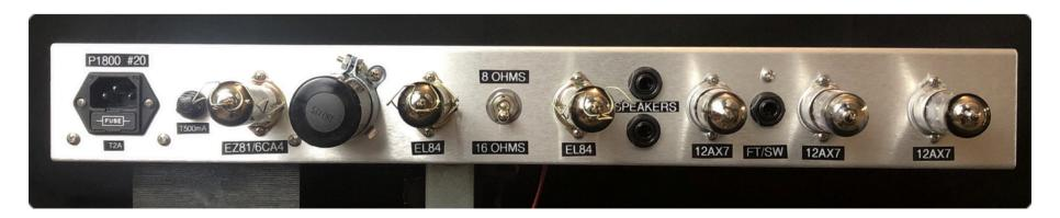
The bottom panel includes the IEC power cord socket (with mains fuse), HT fuse, tube sockets for 6CA4/EZ81, two EL84s and three 12AX7s, impedance selector switch, two speakers jacks and a jack for the footswitch.
